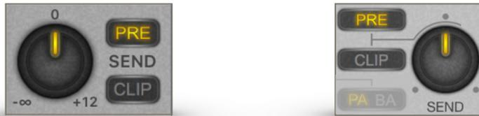
The send volume knob is to set the send amplification of the given port. Along with the state of the PRE button it determines the volume of the signal sent out on the port send output.
