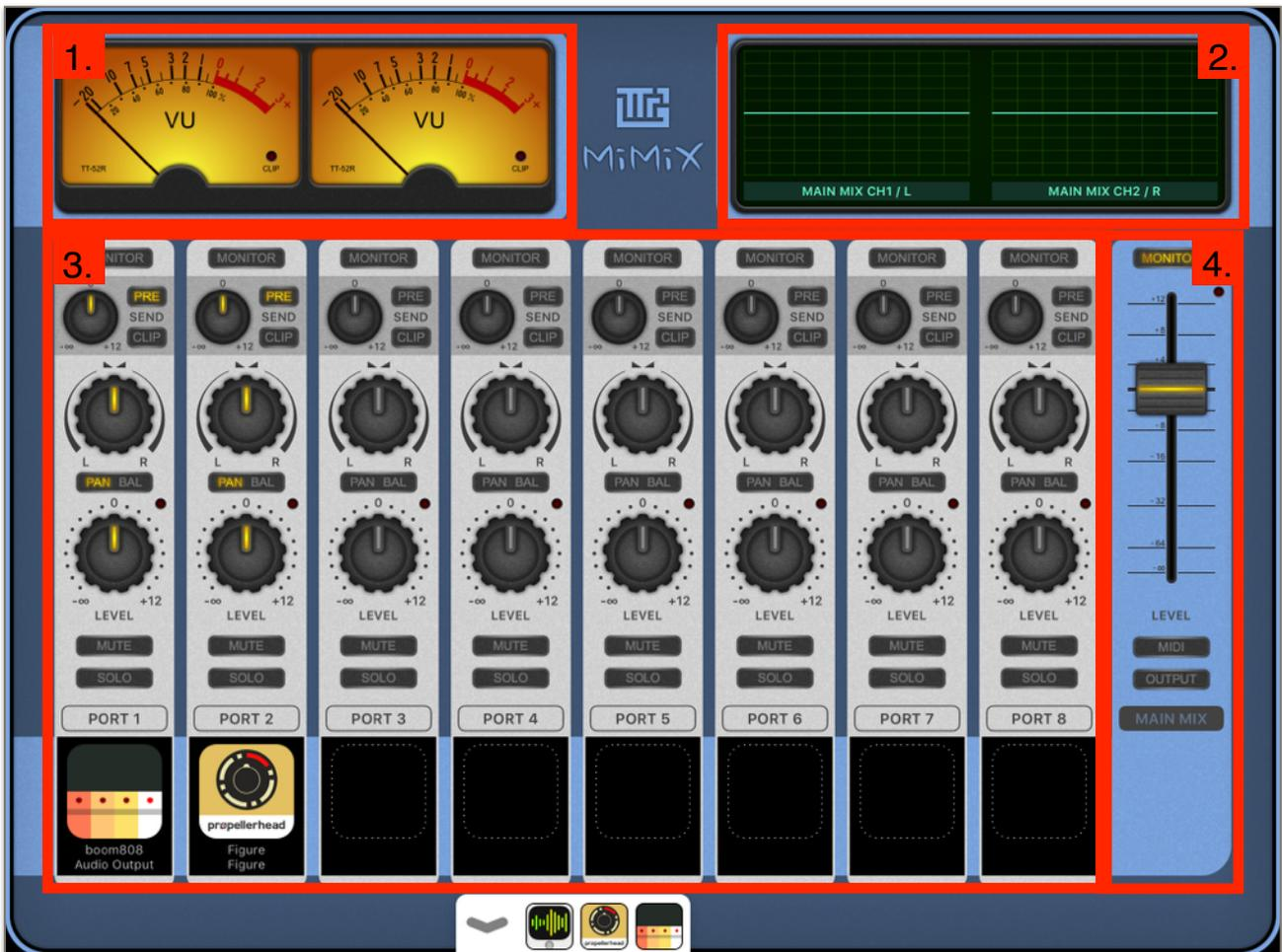
1. The VU meter. This meter will display the power of the signal for the main mix or one port, depending on which is set to be monitored.
