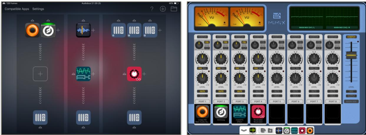
Here, the output of ports 1-3 will go into the FX app and then routed back to MiMiX(mini). This way You can control the wet and dry parts of the mix perfectly. In this scenario the PRE buttons of the send ports should be ON so You can have separate volumes for the dry signal and the one that goes into the FX.
